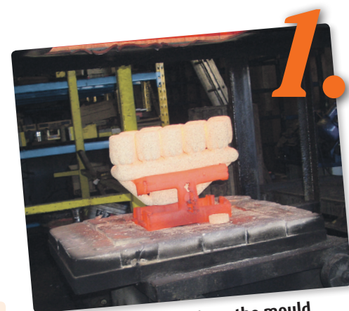
1. Burning out the wax from the mould
