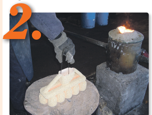
2. Wax burnt out, ready to pour the stainless steel in
