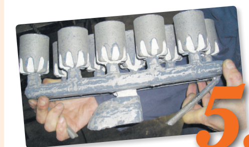
5. Poured mould, cold with ceramic knocked off
