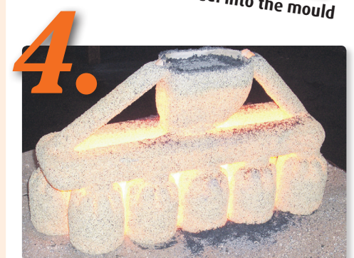
4. Metal poured in the mould but still hot
